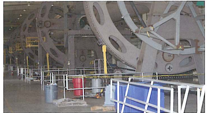
Aker Solutions manufactures umbilicals onsite. Every wheel provides a different element of the umbilical including power and remote control.
