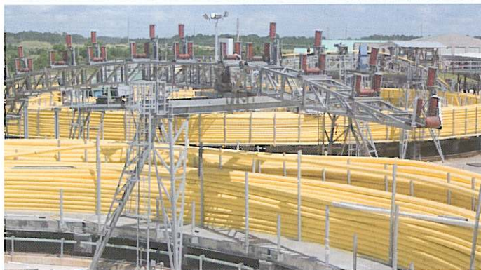
The umbilicals made by Aker Solutions provide power, data, hydraulic functions and chemical injects to underwater drilling sites.
